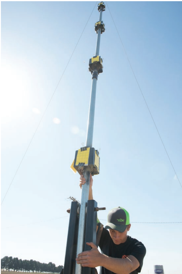
Fig. 1. Insect tower installed outside edge of potato field (Photo credit: Silvia I. Rondon).
